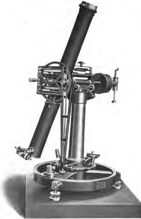
FIG. 35. — A Zenith-Telescope By Warner & Swasey
